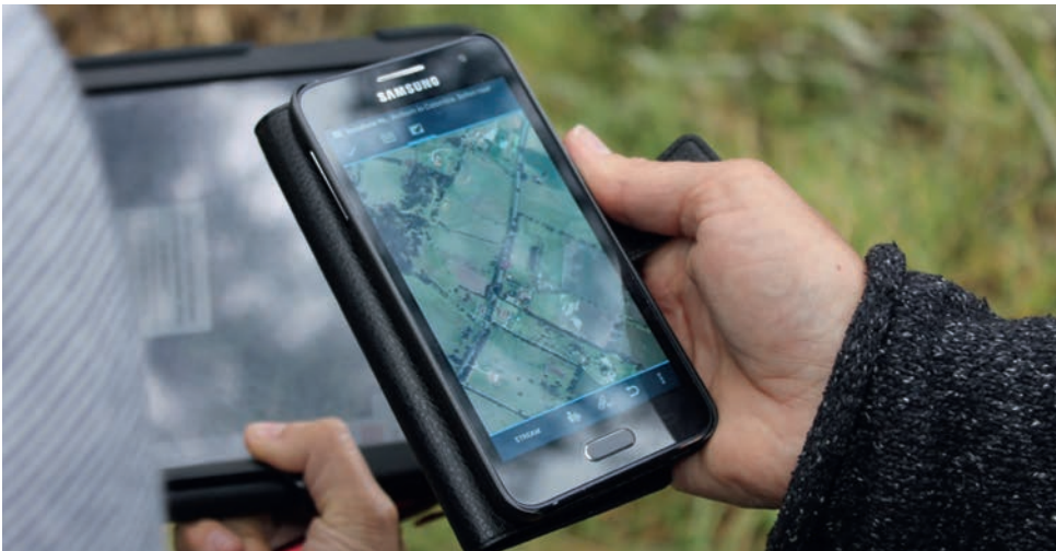
▲ Figure 3, Handheld devices allow cadastral data collection with sub-metre accuracy providing correction signals can be accessed.
