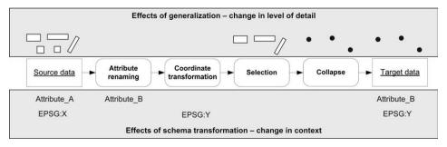
Fig. 5. Processing steps of the content transformation process applied in the presented case study.
