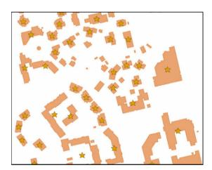
**Fig. 6.** An example map depicting Helsinki building polygons as source data and the symbolized process result (selected and collapsed building geometries).
