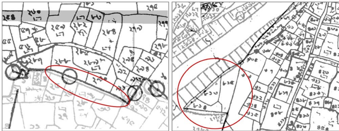
4 Gaps and overlaps in adjoining mouza boundaries (mapping or plotting error)
