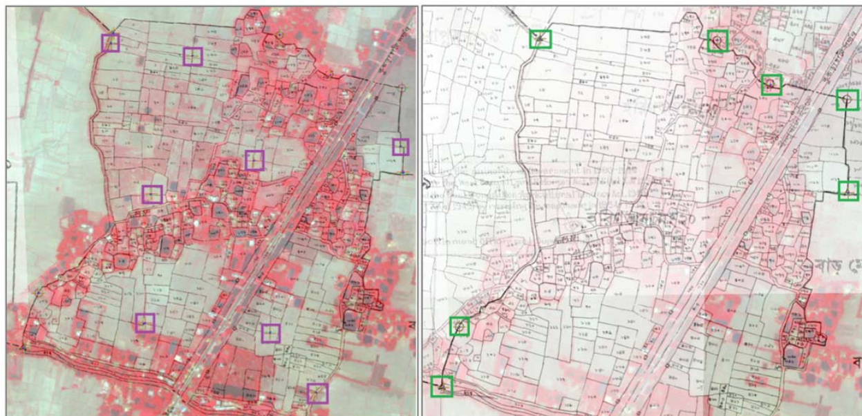
2 Selection of ground control points (GCPs) from image features (L) and by edge matching (R)
