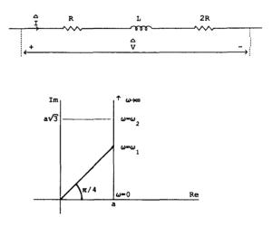
Fig. 4. A simple port and the polar diagram of its complex impedance (cf. Problem 4). The current and the voltage are in complex phasor notation.
