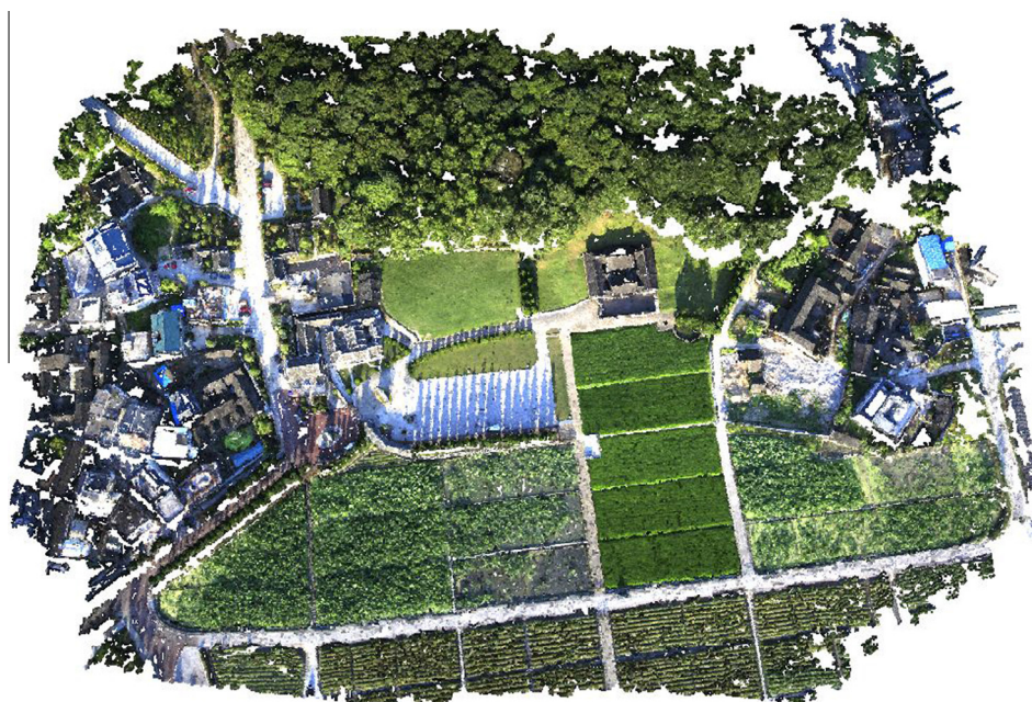
Fig. 15. Dense point cloud with RGB color information of Site B reconstructed by the proposed SCN-SfM method (after densification using PMVS).
