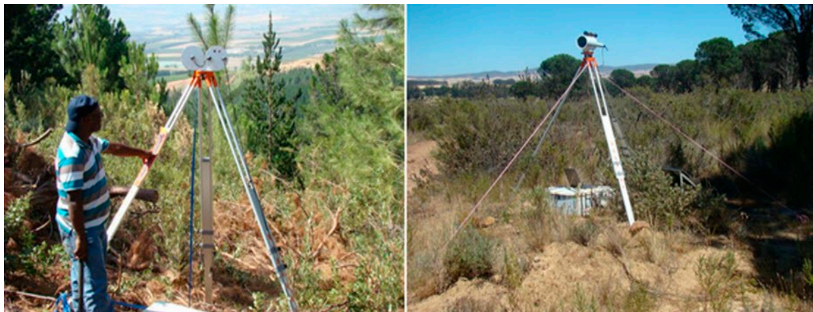
Figure 3. (left) LAS transmitter of infrared radiation; and (right) receiver of the optically modified infrared beam located about 900 m away from the transmitter.
