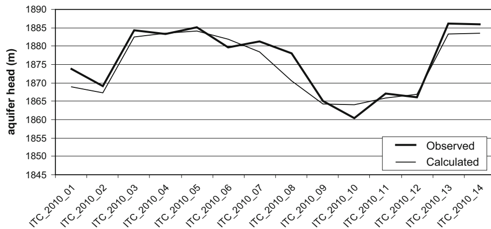
Fig. 9 Observed and calculated aquifer head (observation, June 2010)
