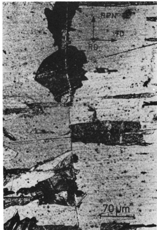
Fig. 9. Photomicrograph of grain boundary area of 49.8% rolled \{112\}\langle 111 \rangle bicrystal annealed for 15 s at 400°C; viewing plane perpendicular to rolling direction.
