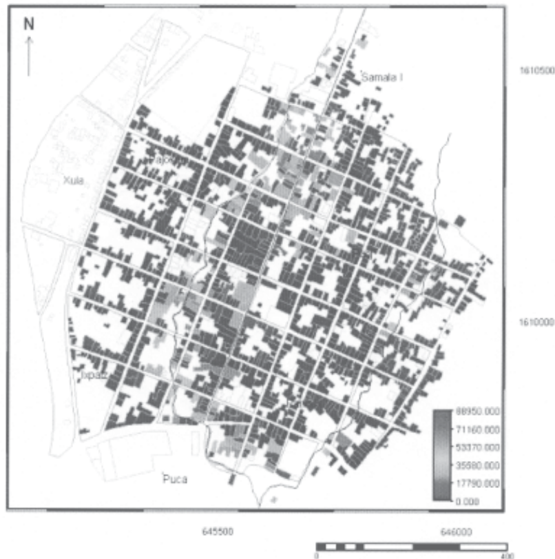
Figure 8 - Map of Total Expected Damage for elements at risk (combined building and content loss). Prices are given in Quetzals (1 USD = approx. 8 Quetzals at the time of this research - October 2002).
