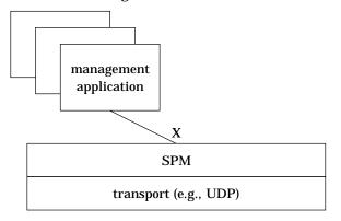
Communication between SPM and management applications uses interprocess communication, such as TLI and sockets. As such, it is even possible to run management applications on different machines. Of course there is a performance penalty in having this multi-process structure with IPC. We believe however that this performance penalty is sufficiently compensated by the improved flexibility and the lower complexity.
