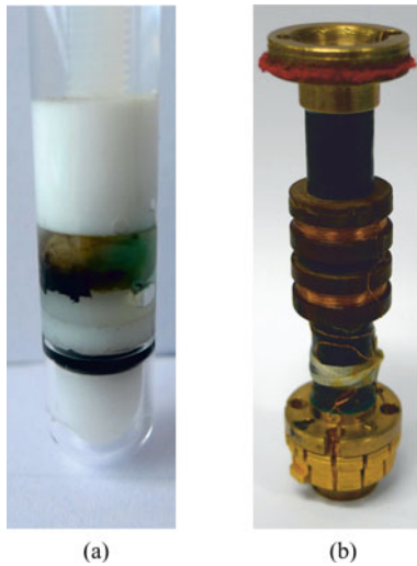
Fig. 1. (a) Lymph node sample fixated with plastic system in glass tube. (b) VSM detection coil set with bore diameter 10.6 mm.
