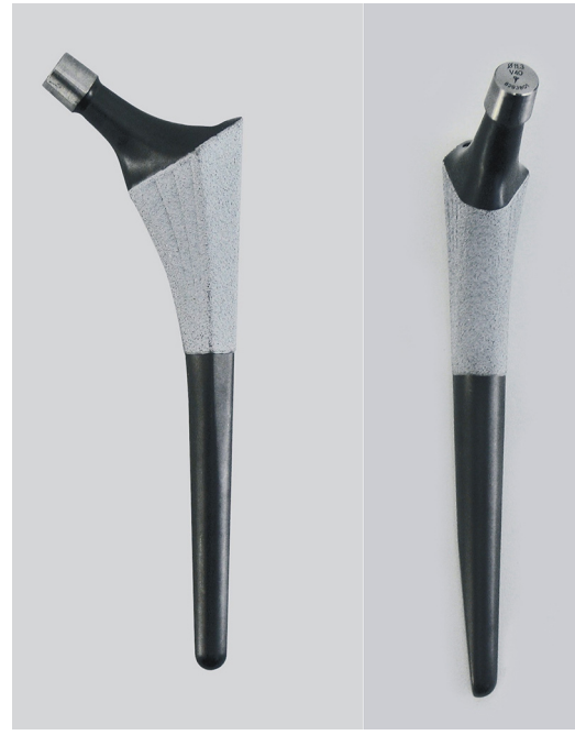
Fig. 2. Illustrations of the Symax ™ stem in AP (left) and lateral (right) view, showing a straight stem with the neck in an anteverted position. It features a proximal plasma-sprayed CP titanium layer, with a biomimetic electrochemically deposited BONIT ® -HA coating of very high porosity of 60%, and only 10–20 \mu\text{m} thick. Distally the stem is treated with the Dotize ® surface process, which reduces distal bone apposition and osseointegration.
