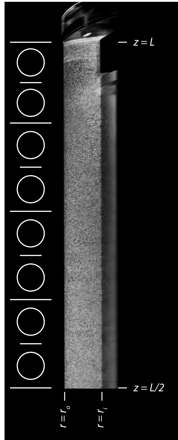
FIG. 9. Visualization of the flow in the top half of the radial-axial plane. The flow is illuminated using a laser sheet in aforementioned plane and photographed from the side using a camera. One can clearly see the pattern of the light streaks visualizing the trajectory of tracer particles. Indications on the left show the placements of the vortex pairs.
