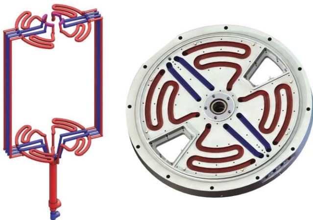
FIG. 5. (Color online) (Left) Schematic sketch of the coolant flow through the T 3 C. Coolant enters at the bottom rotary union (blue) and flows straight up to the top plate by piping on the outside of the TC tank. Then the coolant enters the curling channels in the top plate (red) and is fed downwards again to run through the curling channels of the bottom plate before it exits at the second rotary union. (Right) Bottom plate with the copper cover removed.
