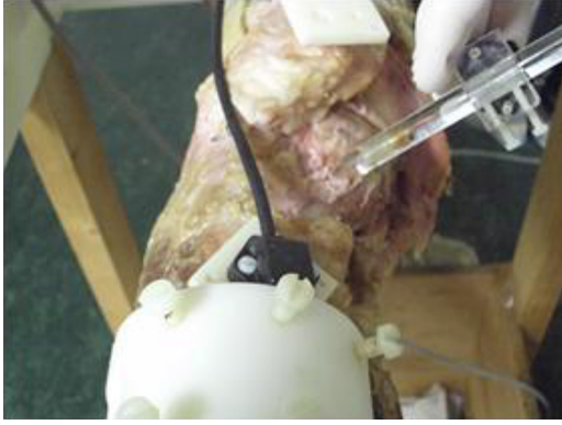
Fig. 3. Collecting registration points using an electromagnetic Fastrak sensor-based stylus of three bony surfaces.
