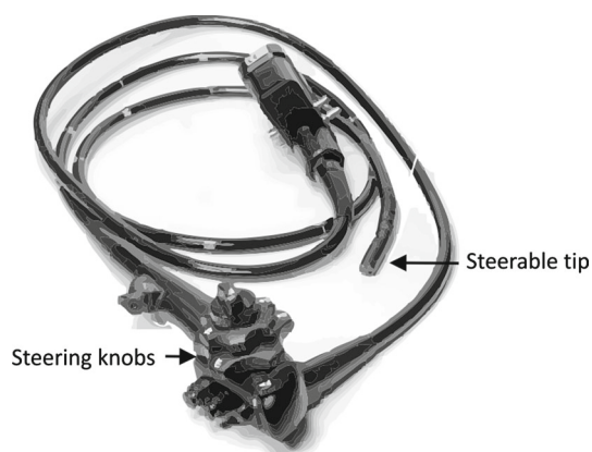
Fig. 1 A typical colonoscope with two steering knobs which are used to steer the tip up/down or left/right
