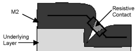
Fig. 11. Modeling of the step-coverage problem of metal layer as resistor.
