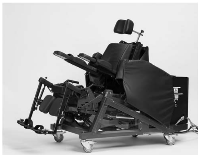
Figure 1 The Dynasit chair, a computer-aided, adjustable simulator chair with parallelogram to control sitting posture.
