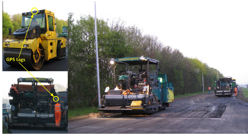
Fig. 8. GPS tags mounted on a roller and a paver (left), data collection site (right).
