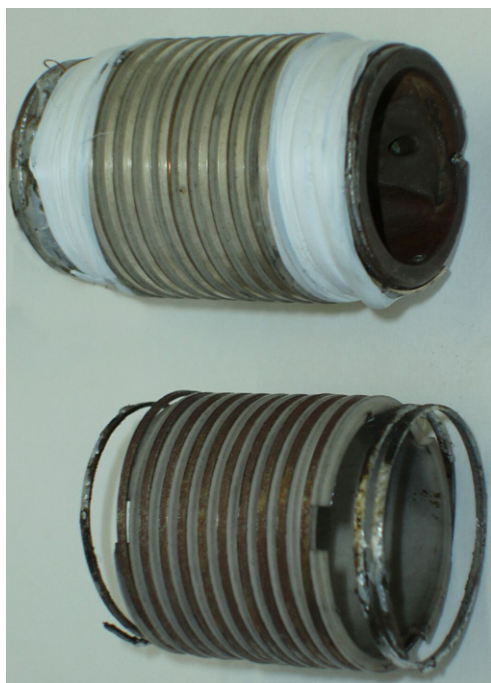
Figure 10. Single-layer helical coils wound of EF and IF wires on the ceramic former of 38 mm diameter and connected to current terminals.
