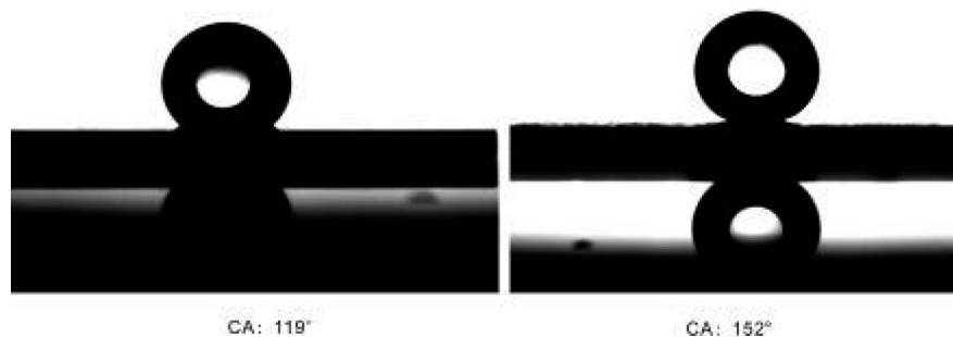
Figure 5. A 5 \mu\text{L} water droplet on OTS SAM modified d1.5p3.5 substrate without (left, CA = 119°) and with 60 nm silica nanoparticles (right, CA = 152°).
