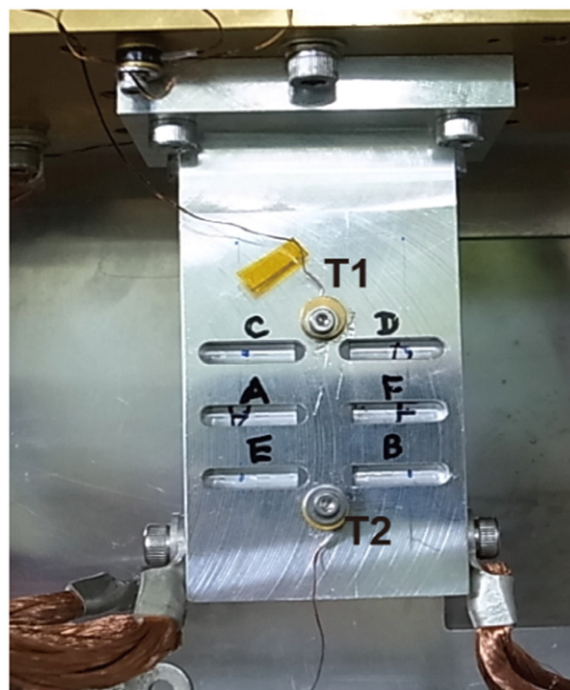
Figure 2. Sample holder for diffraction measurements as a function of temperature. (A)–(F) are slots for samples and (T1), (T2) are temperature sensors.
