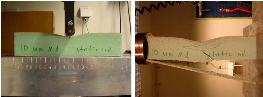
Fig. 2. A sandwich beam of second configuration subject to local indentation (left) and edgewise compression (right).
