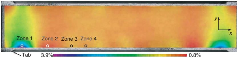
Figure 3. Typical strain field ( \epsilon_y ) in the core prior to the failure. Undeformed coordinate system.
