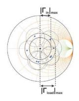
Fig. 9. Matchable area of a 4-bit switchable single circulator based matching network, for  $|\Gamma_{in}| = 1/3$ .
