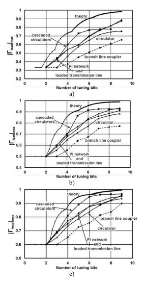
Fig. 12. Magnitude of the load reflection coefficient vs. number of bits for: (a)  $|\Gamma_{in}| = 1/3$ ; (b)  $|\Gamma_{in}| = 1/2$ ; (c)  $|\Gamma_{in}| = 3/5$ .
