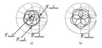
Fig. 21. (a) states enclosing the center of the Smith chart; (b) states enclosing the center of the Smith chart for  $|\Gamma_{out}| = |\Gamma_{in}|$ .
