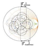
Fig. 5. Matchable area of a 4-bit switchable loaded transmission line based matching network on a Smith chart for  $|\Gamma_{in}|_{max} = 1/3$ .
