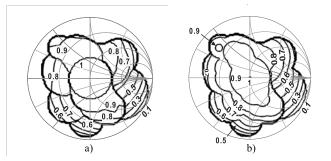
Fig. 18. For a 4b-tunable PI network for  $|\Gamma_{in}|_{max} = 1/3$  in silicon ( $Q_C = 20$ ,  $Q_L = 10$ ): (a) constant power efficiency contours; (b) constant matching efficiency contours for the same case.
