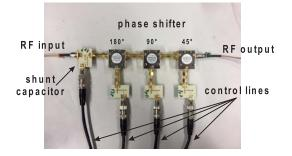
Fig. 14. Photo of the prototype implemented and measured in the lab.
