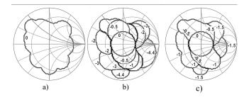
Fig. 22. Available power gain in dB for (a) a lossless 4 bit tunable PI network designed for  $|\Gamma_{in}| \le 1/3$ , (b) a silicon implementation, (c) an implementation in GaAs.
