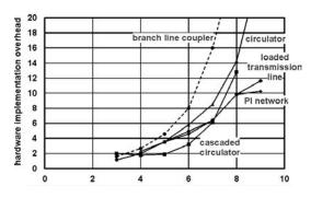
Fig. 13. Hardware implementation overhead versus number of bits for different switchable matching network topologies for  $|\Gamma_{in}| = 1/3$ . For 4, 5, 6, and 7 bit tunability, the cascaded circulator topology has a lower hardware overhead compared to the other switchable matching network topologies.
