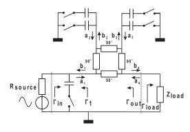
Fig. 6. Implementation of a 5-bit switchable branch line coupler based matching network.
