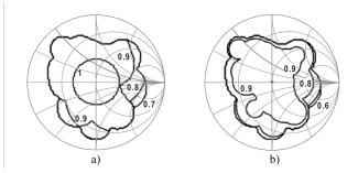
Fig. 19. For a 4b tunable PI network for  $|\Gamma_{in}|_{max} = 1/3$ , implemented on GaAs (Q<sub>C</sub> = 60, Q<sub>L</sub> = 35) (a) constant power efficiency contours; (b) constant matching efficiency contours for the same case.
