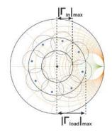
Fig. 11. Matchable area of a 4-bit switchable cascaded circulator based matching network, for  $|\Gamma_{in}| = 1/3$ .
