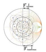
Fig. 3. An example of matchable area of a 4-bit switchable low pass PI matching network based on brute force computing on a Smith chart for  $|\Gamma_{in}|_{max} = 1/3$ .
