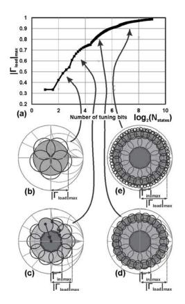
Fig. 1. Minimum number of states matching construction to match from any  $|\Gamma_{load}| \leq |\Gamma_{load}|_{max}$  to within anywhere inside  $|\Gamma_{in}| \leq |\Gamma_{in}|_{max}$ . For  $|\Gamma_{in}|_{max} = 1/3$  this yields the  $|\Gamma_{load}|_{max}(N_{states})$  graph in (a) and example configurations in (b) enclosing the center of the Smith chart and in (c)–(e) having respectively 1, 2, and 3 rings of regions that can be matched to the center circle.
