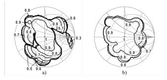
Fig. 20. Constant mismatch contours for a PI network (a) in silicon and (b) in GaAs, showing only the regions where the efficiency with a matching network is better than that without matching network.
