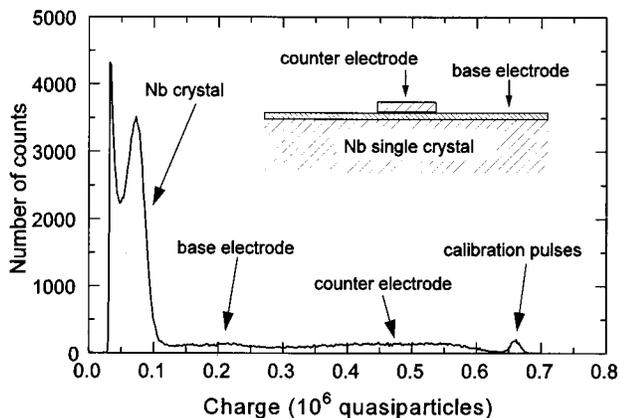
FIG. 4. Pulse height spectrum of  $5.9$  keV x rays, as detected with a superconducting tunnel junction on a Nb crystal.
