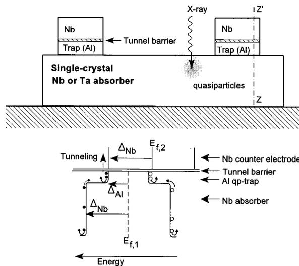
FIG. 1. Schematic representation of the detector concept and quasiparticle potential as a function of vertical position (along a line ZZ' through a junction). The Fermi levels  $E_f$  below and above the barrier are different because of the applied bias voltage.
