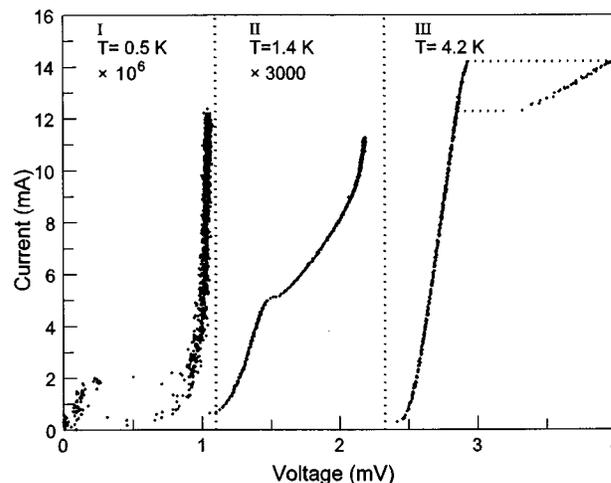
FIG. 2. I-V characteristics of a typical superconducting tunnel junction on a Nb single crystal surface. The area of this junction is 5000  $\mu\text{m}^2$ . Note that the current scales and temperatures  $T$  differ in the three regions.
