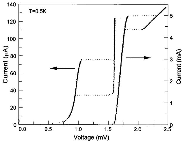
FIG. 3. I-V characteristics at  $T=0.5$  K of a superconducting tunnel junction on a Ta single crystal surface. The area of this junction is  $5000 \mu\text{m}^2$ .
