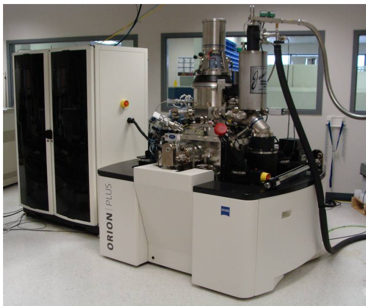
FIG. 1. The completed NUHV Helium Ion Microscope
