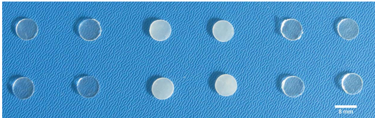
Fig. 5. \phi 8 mm PTMC discs (left 4), PTMC discs with GEN-SULPH (middle 4) and PTMC discs with GEN-AOT (right 4) prepared by compression molding.
