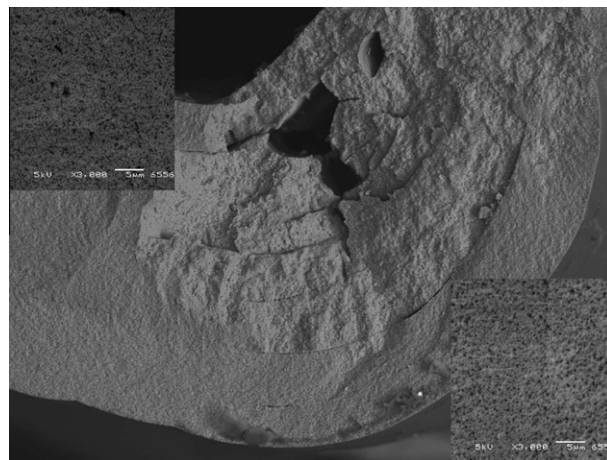
Figure 1. Scanning electron microscope microstructures of sintered sample D15: cross-section with eight layers, inner surface with high porosity (up), outer surface with low porosity (down).
