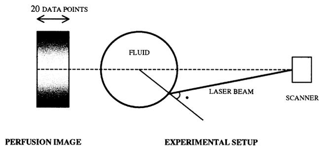
Fig. 1. Experimental design to investigate the effect of tissue curvature in vitro. The laser beam scans the surface with underlying fluid and a rectangular perfusion image is formed. Incident angles are calculated from the position of the measurement site in the image. A similar design is used in vivo, where the fluid is replaced with the subject's forearm.
