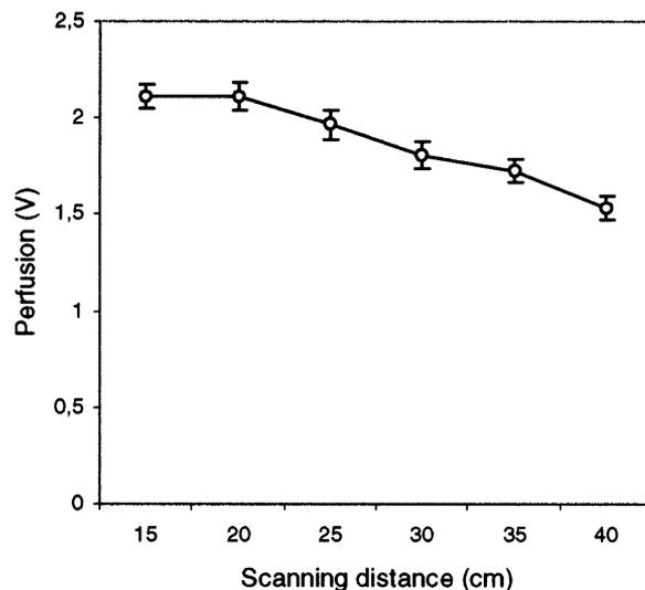
Fig. 2. The effect of scanning distance on the perfusion signal, as measured in vitro.
