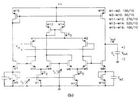
Fig. 1. (a) OTA proposed in [9]. (b) Modified OTA using stacked square-law transistors.
