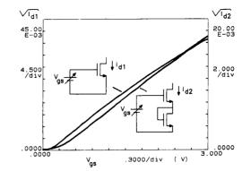
Fig. 2.  $\sqrt{I_d}$  versus  $V_{gs}$  of a single 50/10 NMOS transistor compared to a stacked pair of 50/10 NMOS transistors: the stacked pair has a better square-law behavior for  $V_{gs} = 0.6-3$  V.
