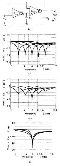
Fig. 3. (a) Second-order notch filter. (b) Frequency characteristics of the filter for  $V_0$  tracking  $V_c$  according to  $(V_c - V_{Teq})/(V_0 - V_T) = 3.2$ . (c) Idem for a constant  $V_0 = 0.64$  V. (d) Idem for constant  $G_{m1}G_{m2}$  and Q = 0.5, Q = 1, and Q = 2.
