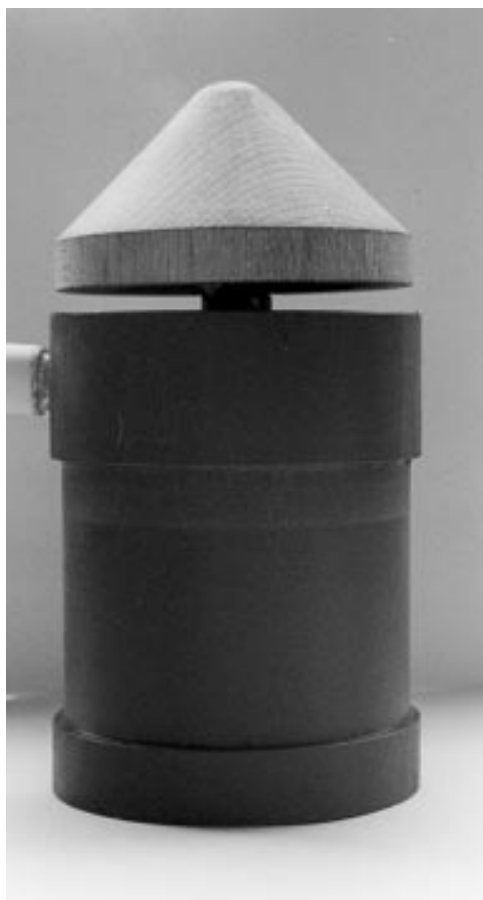
Figure 3 Modified indenter with central load washer.
