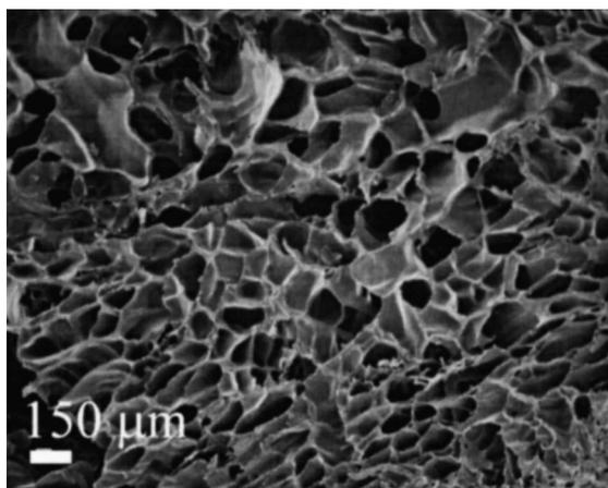
Fig. 5. Porous structures of 1000 PEOT70PBT30 prepared by freeze-drying (solid–liquid phase separation of 10% dioxane solutions). Freezing temperature:  $+6^{\circ}\text{C}$  (pore size  $\pm 125 \mu\text{m}$ ).
