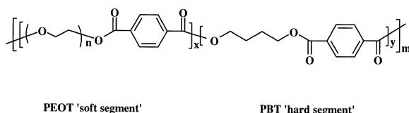
Fig. 1. Chemical structure of PEOT/PBT segmented block copolymers.
