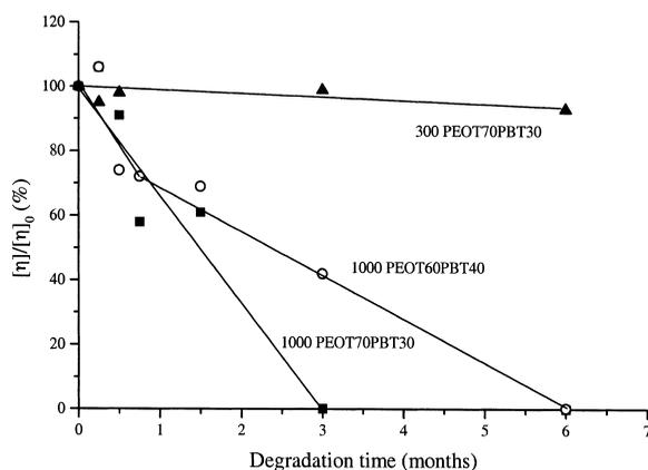
Fig. 4. Relative intrinsic viscosity ( $[\eta]/[\eta]_0$ ) during degradation in PBS at 37°C for 1000 PEOT70PBT30 (■), 1000 PEOT60PBT40 (○) and 300 PEOT70PBT30 (▲).
