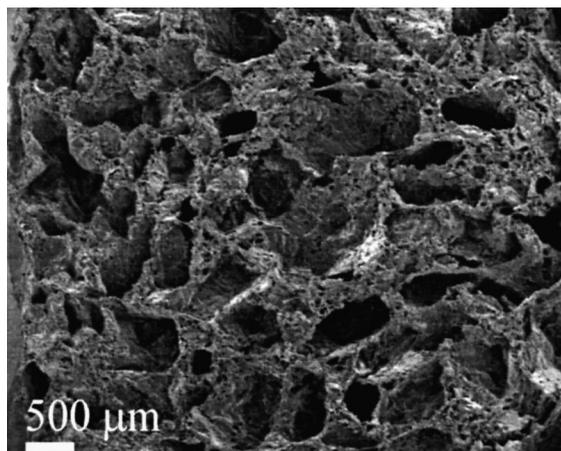
Fig. 6. Highly porous structures obtained by combination of freeze-drying (freezing temperature:  $-28^{\circ}\text{C}$ , pore sizes: 70–90  $\mu\text{m}$ ) and salt-leaching (pore size: 400–700  $\mu\text{m}$ ). A 10%-solution of 1000 PEOT70PBT30 in dioxane containing sucrose crystals was used; the overall porosity is 94%.
