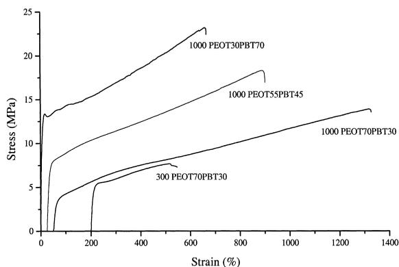
Fig. 2. Stress-strain diagrams of PEOT/PBT block copolymers of different compositions (measurements performed on dry specimens). Stress-strain curves are offset for clarity.
