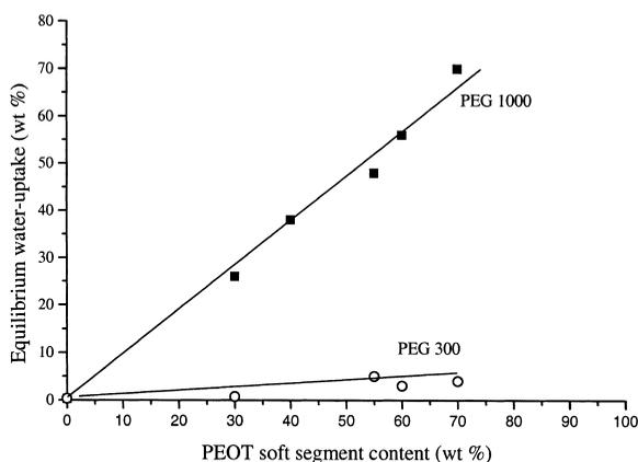
Fig. 3. Equilibrium water-uptake (wt%) as a function of PEOT soft segment content (wt%) for PEOT/PBT copolymers synthesized from PEG 1000 (■) and PEG 300 (○).
