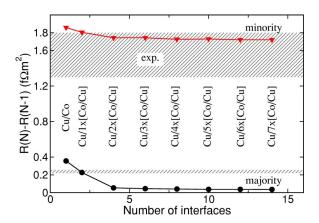
FIG. 13. (Color online) Differential interface resistance as the number of interfaces increase for a disordered Cu(10ML)/Co(10ML) multilayer embedded between Cu leads. A  $10\times10$  (111) lateral supercell was used and the interface was modeled as two layers of 50%–50% alloy (2ML model). The results represent an average over five disorder configurations and were obtained for a "standard" configuration (Ref. 63). The range of experimental values (Ref. 76) is indicated by the shaded regions.
