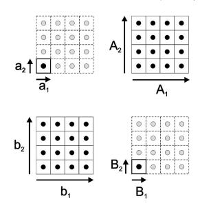
FIG. 2. Illustration of lateral supercells and corresponding 2D interface Brillouin zones. Top panel: lattice vectors for a primitive unit cell containing a single atom [left-hand side (lhs)] and a  $4 \times 4$  supercell [right-hand side (rhs)]. Bottom panel: a single k-point in the BZ (rhs) corresponding to the  $4 \times 4$  real-space supercell is equivalent to  $4 \times 4$  k-points in the BZ (lhs) corresponding to the real-space primitive unit cell.
