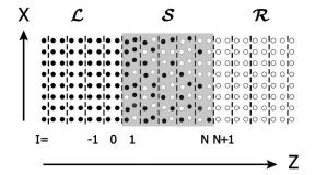
FIG. 1. Sketch of the configuration used in the Landauer-Büttiker transport formulation to calculate the two terminal conductance. A (shaded) scattering region ( $\mathcal{S}$ ) is sandwiched by left- ( $\mathcal{L}$ ) and right-hand ( $\mathcal{R}$ ) leads which have translational symmetry and are partitioned into principal layers perpendicular to the transport direction. The scattering region contains N principal layers but the structure and chemical composition are in principle arbitrary.
