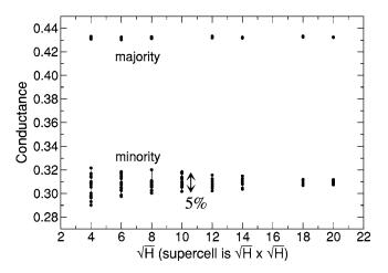
FIG. 7. Interface conductance (in units of  $10^{15} \Omega^{-1} \text{ m}^{-2}$ ) for a disordered Cu/Co (111) interface modelled as 2ML of 50%-50% alloy in a  $\sqrt{H} \times \sqrt{H}$  lateral supercell as a function of  $\sqrt{H}$ . The results are given for different randomly generated configurations of disorder (15 for minority spin, 5 for majority spin). Results are for a "standard" configuration (Ref. 63).
