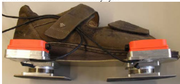
Figure 1. Instrumented shoe with two force transducers and inertial sensors (in orange attached to the transducers).
