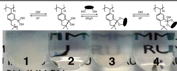
Figure 2. A schematic representation of the polymer 7 with monosaccharides in different pH environments. The photograph shows tubes containing the polymer 7 in different buffers after 18 h. Tube 1: 7 in PBS (pH = 7.4), 2: in PBS/D-fructose (50 mM), 3: in PBS/D-glucose (100 mM), 4: in TRIS/D-glucose (100 mM, pH = 7.8).
