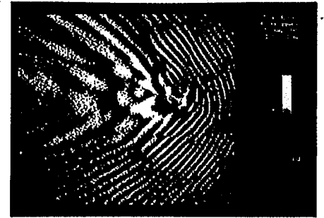
Fig. 5: 11.2 \times 11.2 \mu\text{m} image of a \phi 91 \text{ nm} latex sphere with laser beam incident from right to left scanned at constant height.
