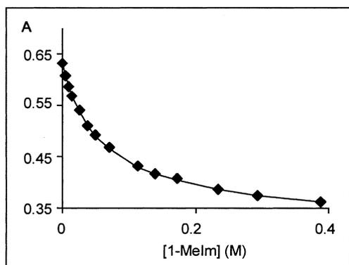
**Figure 9.** Spectral evolution of a 1:1 mixture of porphyrin **1a** and calix **2** in MeOH ( $4 \times 10^{-5}$  M, assembly **1a·2** present >95%) titrated with 1-methylimidazole (1-MeIm). The lower part shows the fitting of the titration curve at 555 nm.
