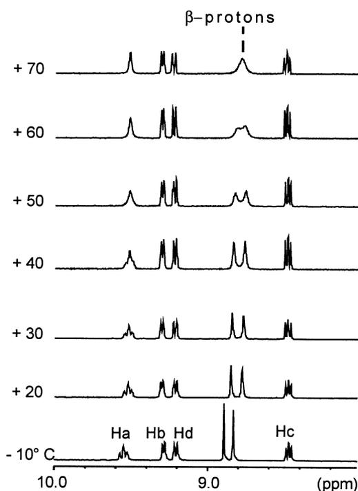
**Figure 2.** VT <sup>1</sup>H NMR experiments of porphyrin **1a**. Experiments were performed using 1.6 mM samples in CD<sub>3</sub>CN/D<sub>2</sub>O (6.5:1.5). Proton assignment as in Fig. 3.
