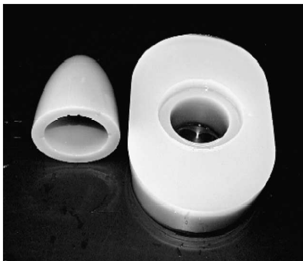
Fig. 2. Left ventricular (LV)-phantom which consists of two parts. The actual LV shaped part is shown on the left and the assisting part is shown on the right of the picture. Both parts are made from agar with carborundum as scattering particles. The assisting part contained a stirring device to assist a homogeneous distribution after UCA injection.
