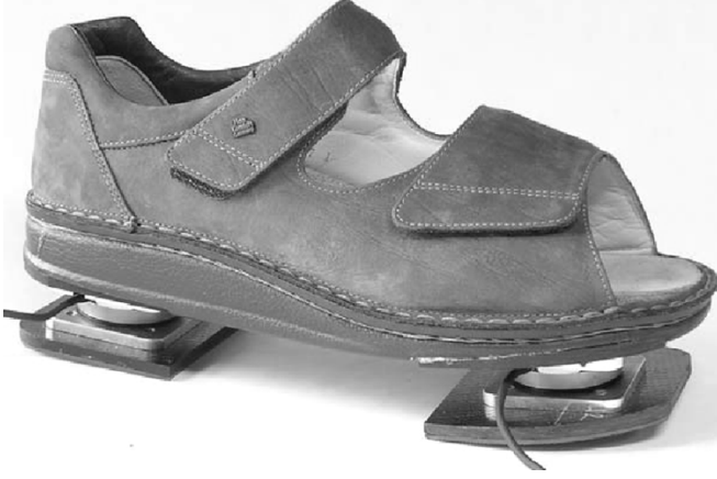
Fig. 1. Shoe instrumented with two 6-axis force and moment sensors.
