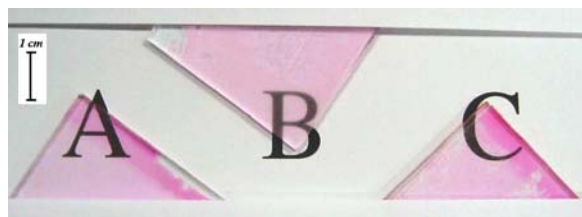
Figure 1. Modifications in the film appearance after washings with water/acetone. (See text for details). The samples shown are: (A) wH-Me-TIP, (B) wH-Me-P-TIP and (C) wH-Me-O-TIP.
