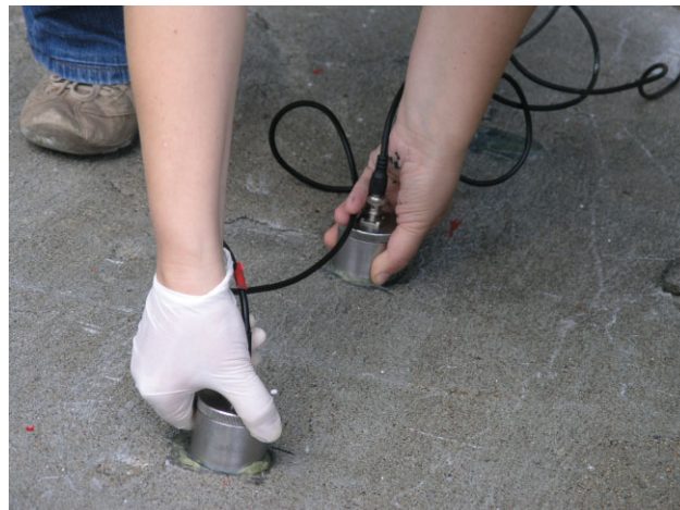
Figure 3. Pulse velocity measurements of the concrete
