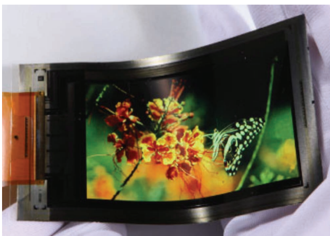
Figure 1. 3.4 inch flexible AMOLED Display with 326 pixels per inch and a total thickness of 50 \mu\text{m} . Reproduced with permission. [177] Copyright 2011, The Japan Society of Applied Physics.
