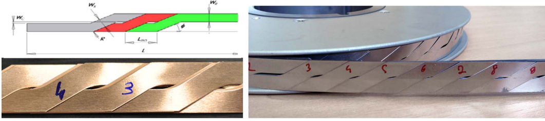
Fig. 5. Roebel cable concept (left); a first 15 tape Roebel cable manufactured by KIT for preliminary EuCARD2 investigation (right).
