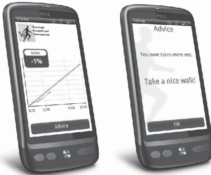
Figure 4: The activity coach running on a HTC Desire (Android 2.2), with on the left: continuous feedback in the form of the activity graph displaying the measured activity (blue) and reference activity (green). The status panel shows the deviation from the reference line. On the right an example of a feedback text message is shown.
