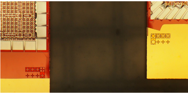
Fig. 10. Microscope image of the SU-8 structures used for the shear test. These structures serve as alignment markers during the wafer post-processing. Note the SiRN layer (red) extending under the markers on the left chip. The adhesion there is a lot stronger than on the gold layer on the right. Also visible are the different support ridge layouts. (For interpretation of the references to colour in this figure caption, the reader is referred to the web version of this paper.)
