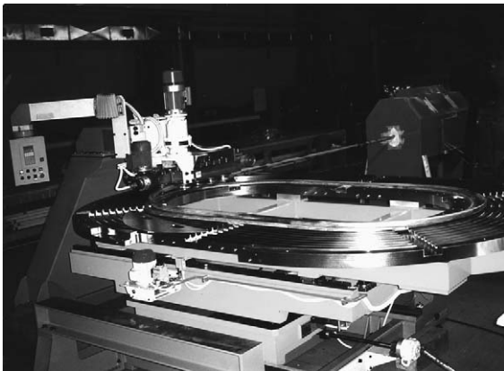
Fig. 3.4. Winding of a pancake into a reaction mould.
