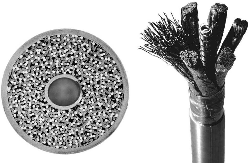
Fig. 3.3. Cross-section and build-up of the TFMC conductor.
