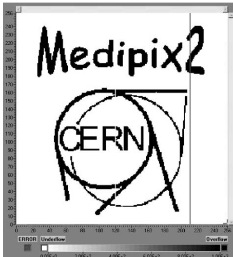
Fig. 4. Screen capture from Medisoft4 software after using MUROS2 to load a mask into a Medipix2 chip, applying test pulses to the selected pixels and reading out the values. The black pixels have 1000 counts and the white 0. The threshold was approximately 4000 electrons and the input charge per event was about 8000 electrons.
