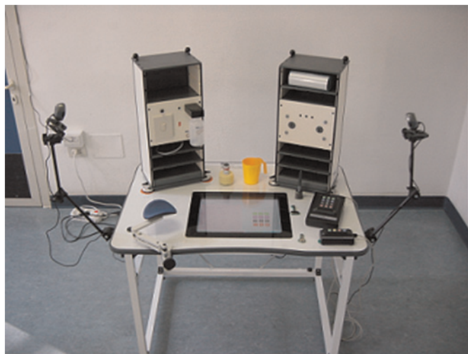
Figure 2 PU with sensors and main variables acquired
