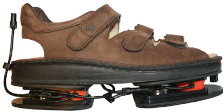
Fig. 1. IFS (right shoe). Each force shoe (left and right) has two sensors modules: one under the forefoot and one under the heel. Sensor module includes a force/torque sensor and a motion tracker.
